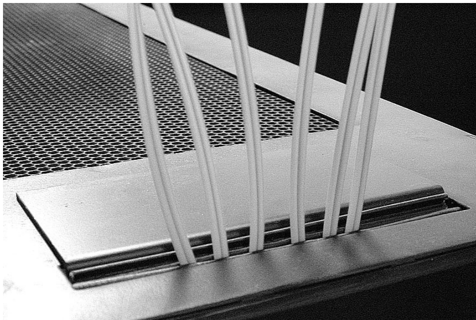
Figure 24. Positioning the Fibre Channel cable outside the frame
